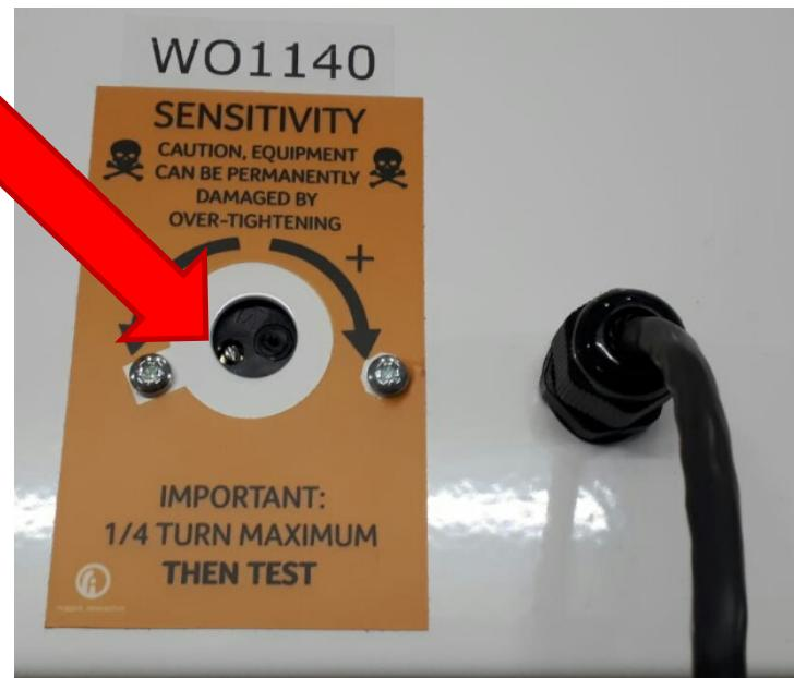
**Figure 3.4.7: Location to adjust the sensitivity**
