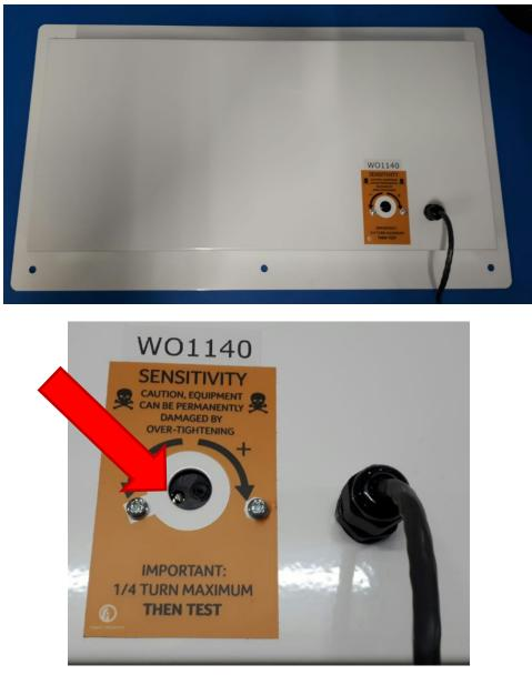
Figure 3.4.7: Location to adjust the sensitivity
