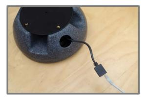
Connect appropriate length CAT5 cable to the start button's hanging cable that will return to the control box. The start button must be within 30m of the control box.
