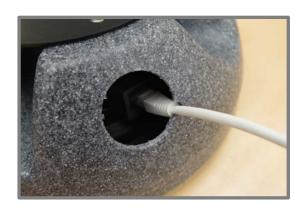
Tuck the hanging cable and head of the CAT5 cable inside the recess in the moulding. Cable excess can be fed into this recess too.
